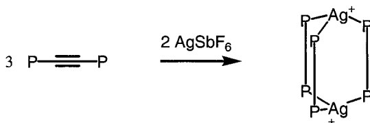
Figure 5. Selective formation of [\text{Ag}_2(\text{dppa})_3]^{2+} complexes at the appropriate metal to ligand ratio.
